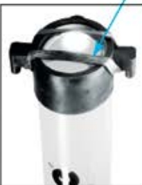
Rubber band prevents balls from falling out
